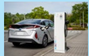
eLINK, a V2X bi-directional charging system enabling the supply of electricity stored in EVs to buildings and other locations (2013)
