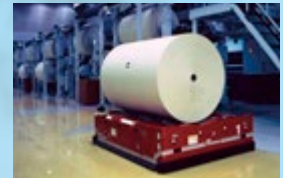
Automatic guided vehicle (AGV) paper feeding system, which has contributed to the automation of newspaper roll conveyors and the improvement of operations (1996)
