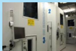
Labostocker 150, a small refrigerated storage system for new drug discovery that is the first in the world capable of storing items at temperatures lower than -150°C (2016)
