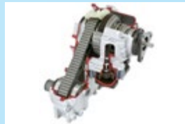
Power Drive Chains for four-wheel drive vehicles, a new automotive parts product (1997)
