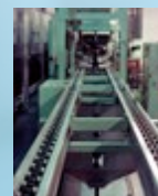
Plastic side roller chain developed for free flow conveyors (1981)
