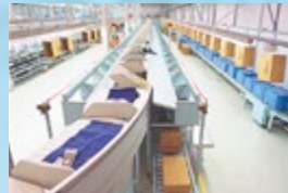
Linisort, linear motor drive automated sorting equipment (1992)
