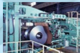
Automated coil packaging system that contributed to labor savings on packaging lines (1976)
