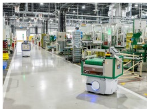
Advancing unmanned operations using small AGVs at our new tensioner factory
