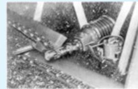
C-60 class chain for use at coal faces helped boost coal production (around 1930)
